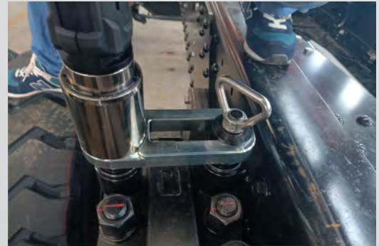
Sliding Reaction Arm
